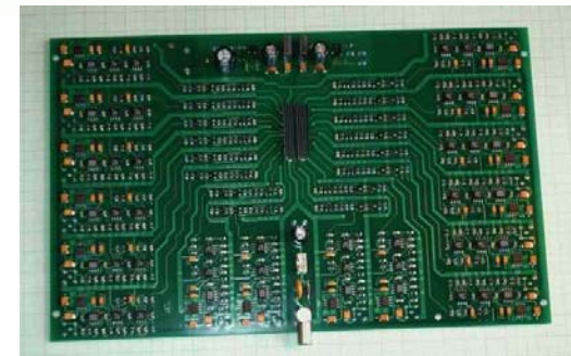
PCB with 16 ch. voltage preamp.
