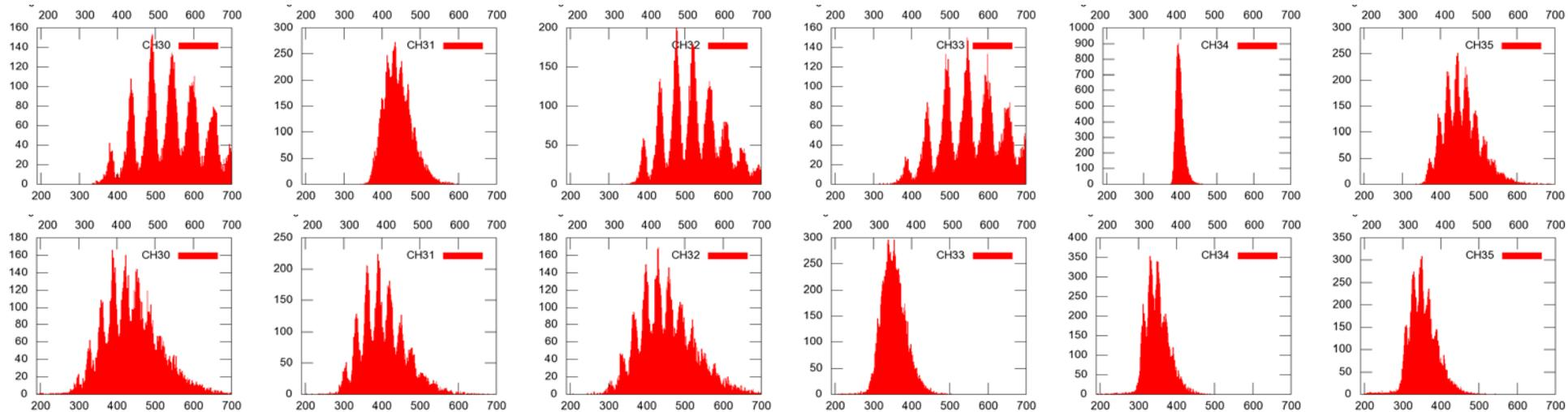
Spread of SiPM gain is about factor 3, it corresponds to data from ITEP.
