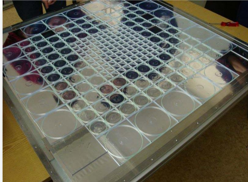
1m3 prototype calorimeter with 8000 channels readout with SiPM
