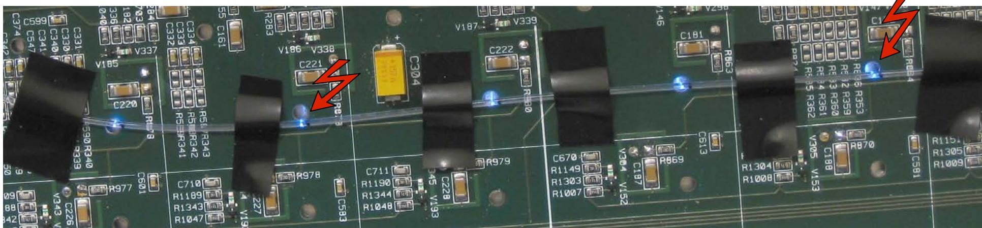
A "NEW" BALSAwOOD bar with a notched fibre Apr 2010
