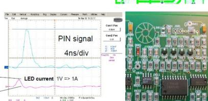
2012 / 2013 we are developing 3 versions of QMB with 1 ns, 5 ns and long pulse 30 ns. Long pulse version is coming with external toroidal inductor.
