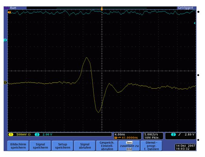
View of the LED pulse for a middle amplitude (1.0 A)
