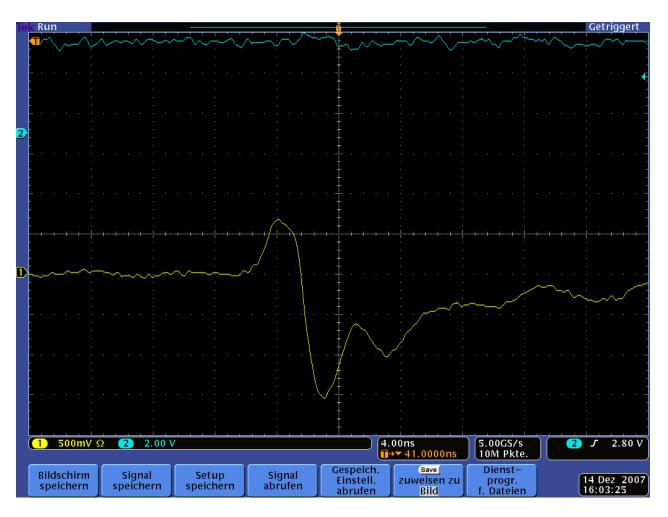
View of the LED pulse for a small amplitude (0.6 A)
