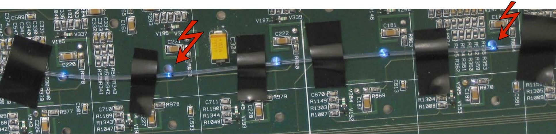
Electrical tape did not fix the bent fiber properly
