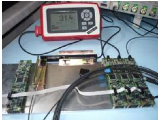
Output optical power vs V1 setting, QMB1, optical fibre 7m in length, 1mm in diameter,
