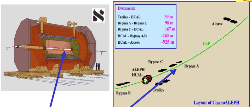
16 m<sup>2</sup> TPC, array of 5 scintillators, experiment running with respect to beam crossing frequency => 11 % duty cycle. Also dedicated runs without beams in accelerator (CosmoALEPH trigger from HCAL)
