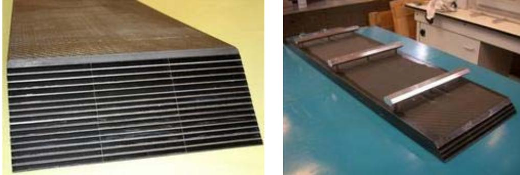
Figure 26: View of the alveolar structure of the EUDET ECAL mechanical prototype
